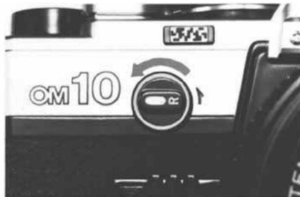
① Turn the rewind release lever when the film ends.
